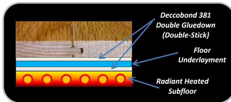
The floor underlayment is a thin layer of material (polyfoam, cork, rubber) that serves to smooth out the imperfection of the subfloor and a cushioning layer between the subfloor and the engineered hardwood floor. Additional functions of the floor underlayment include added comfort to walking, vapor barrier, and sound deadening layer depending on the applications and specifications for multi-residential and multi-commercial dwellings.
